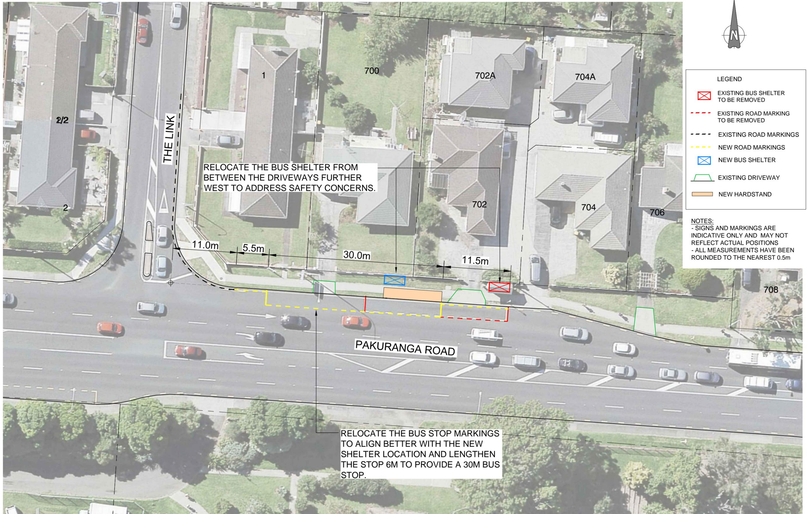
RELOCATE THE BUS SHELTER FROM BETWEEN THE DRIVEWAYS FURTHER WEST TO ADDRESS SAFETY CONCERNS.
