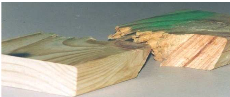
Fig. 8: The plane-failure in a margin knot.
