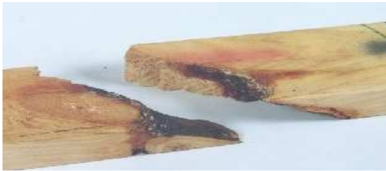
Fig. 7: The boundary-failure in a through arris knot.
