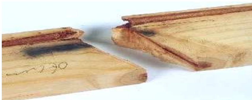
Fig. 9: The plane-failure in an edge knot.
