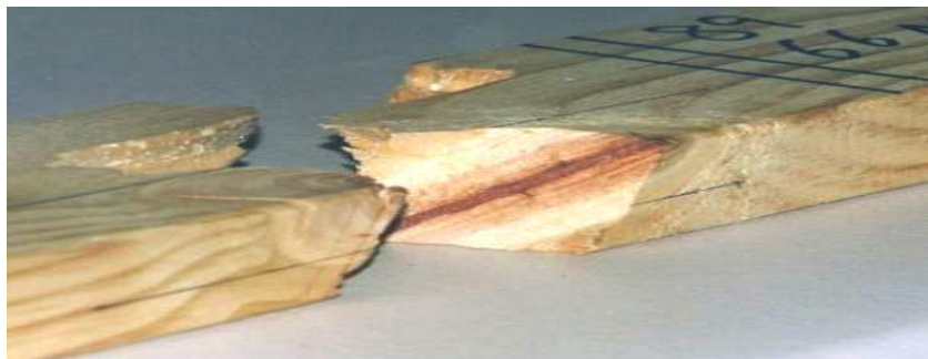
Fig. 10: The plane-failure in a through arris knot.
