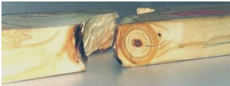
Fig. 6: The boundary-failure in an edge knot.
