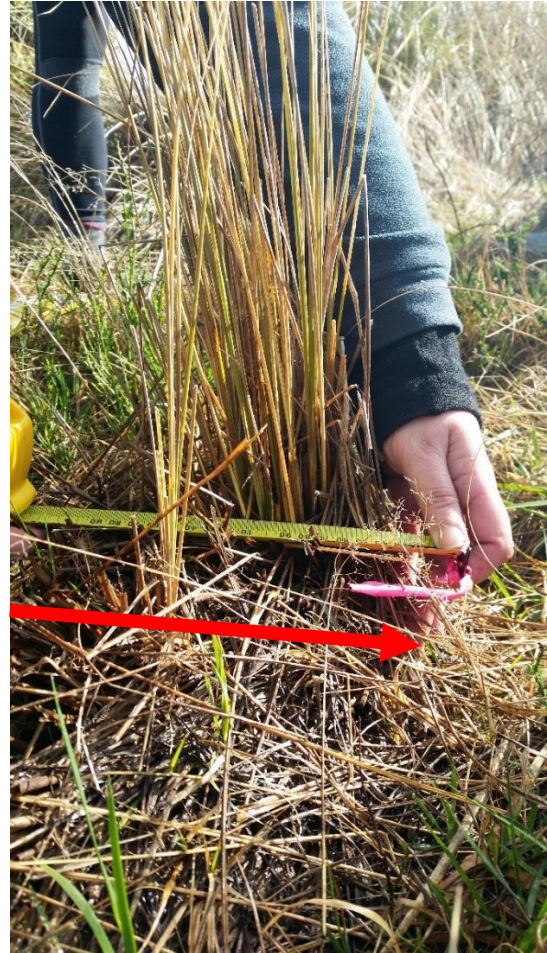
Figure 15. This is the second orthogonal measure taken at right angles to the one shown in Figure 14. Measure across the base, include live and dead tillers until the tussock becomes “botanically indistinct” (shown in a red arrow , at approximately 22 cm here).
