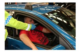
Upon obtaining a result, always point the device away from you/your vehicle and equipment while it automatically purges. Always consider the wind direction.
