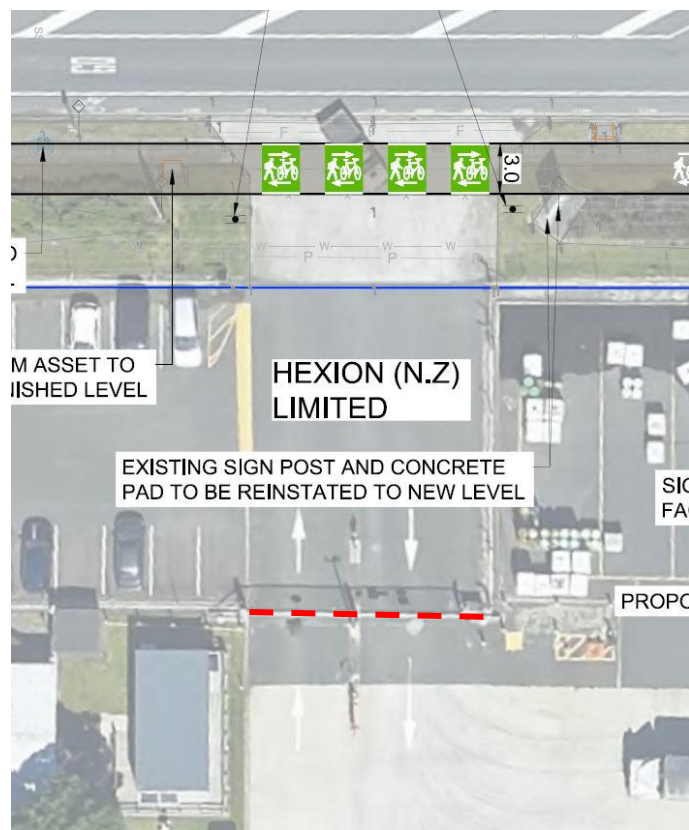
Figure 7: Hexion driveway layout, with gate indicated in red dashed line
