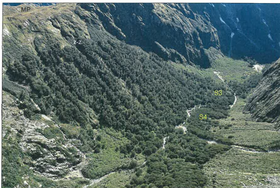
Figure 10 Aerial view of potential hut sites 3 and 4 looking down the Clinton Valley below Mackinnon Pass (MP). The zig-zag (z-z) section of the Milford Track below the pass traverses an old rock fall deposit on the northern side of the valley. Both sites are located in bush near the centre of the valley and are outside the main rock fall zone (left) and the known avalanche paths (Zig-zag and Mintaro, Figure 7). Site S4 is also outside the potential flood zone and debris fan (lower right).
