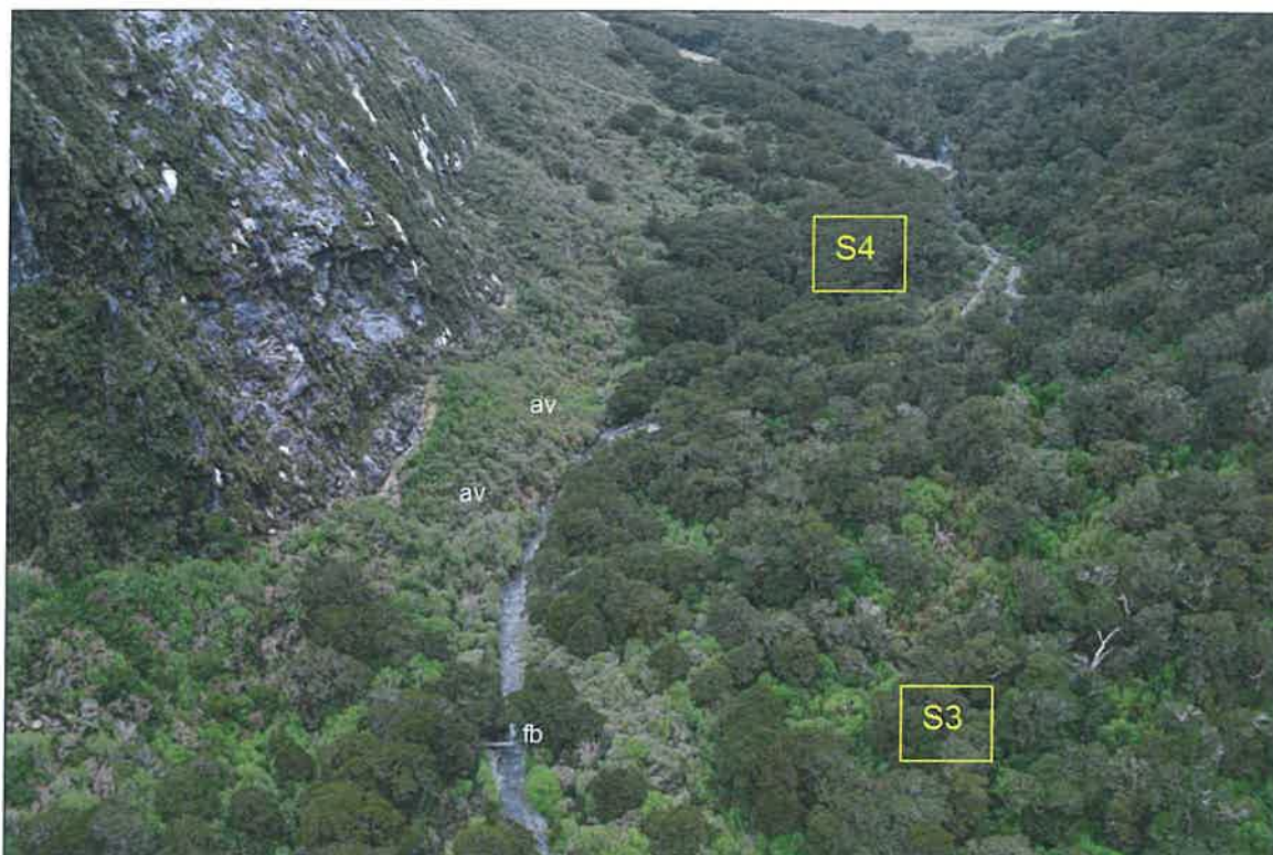
Figure 11 Aerial view looking up the Clinton River towards potential hut Site 3 and Site 4. Site 3 is in an area of large beech trees (dark green) and ribbonwood and fuchsia forest (lighter green). Site 4, which is located in thick beech forest ~250 m upstream from the footbridge ( fb ), is outside the known rock fall, debris flow, flooding, and snow avalanche hazard zones in the area.
