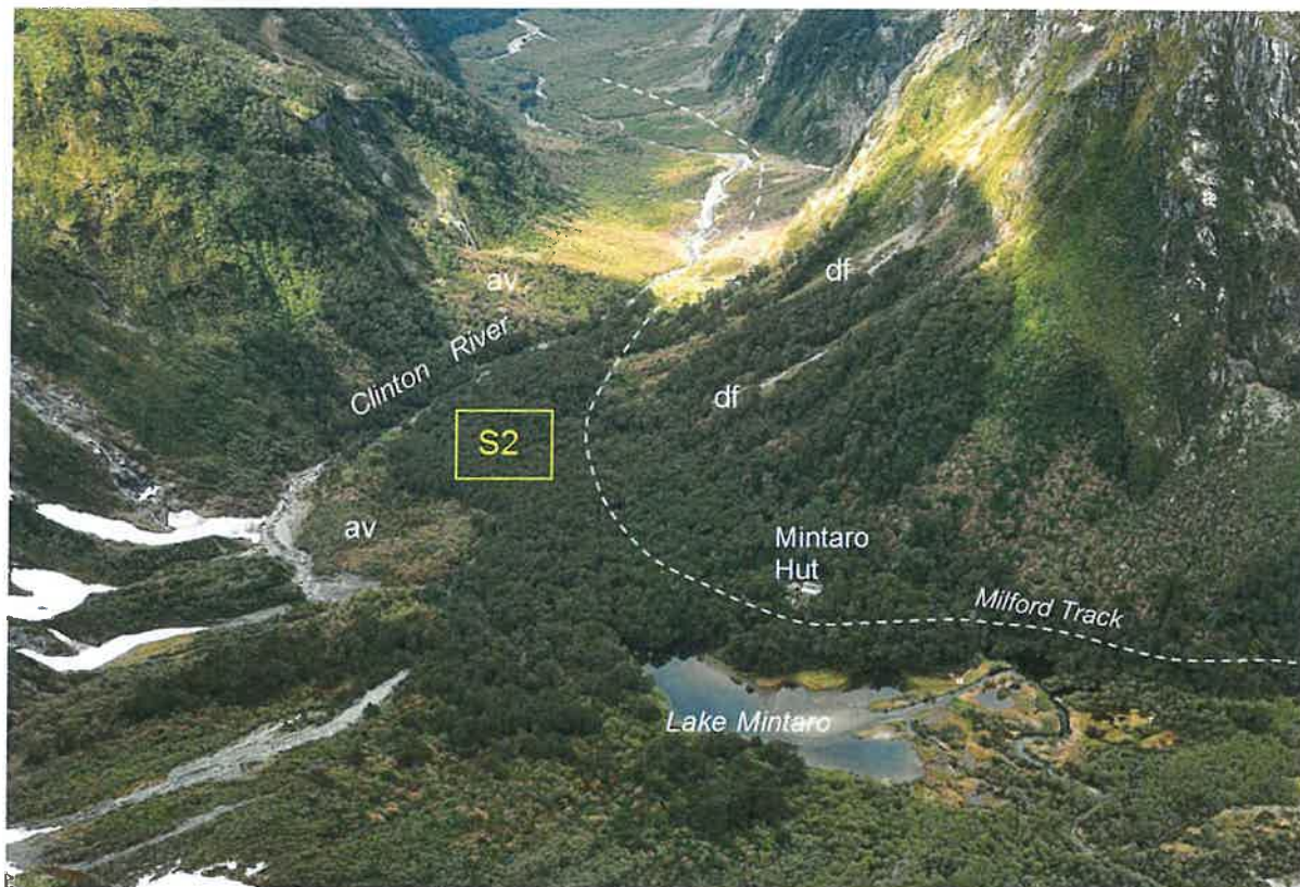
Figure 5 Aerial view of potential hut Site 2 (S2) located in beech forest on the true right left (west) side of the Clinton River, about 500 m down valley from Mintaro Hut. Although the site is generally clear of the avalanche blast zones on the east side of the valley ( av ) and debris flow paths on the western side ( df ), the site and general area is littered with old rock fall boulders under the bush cover.
