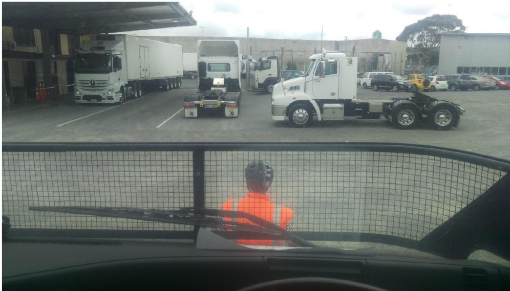
Figure 2: Example of reduced view of cyclist positioned in front of a heavy goods vehicle 2
