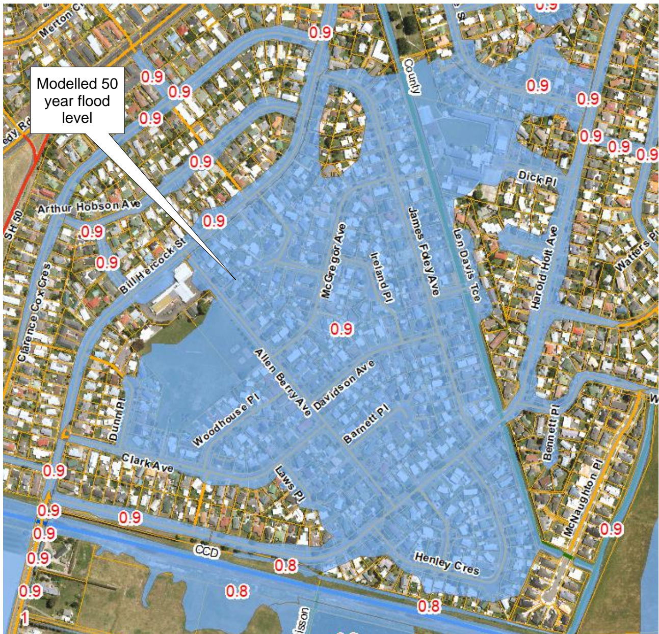
Figure 53: Modelled 50-year return period flood extents in Pirimai (datum NZVD16) (HBRC 2003 model)
