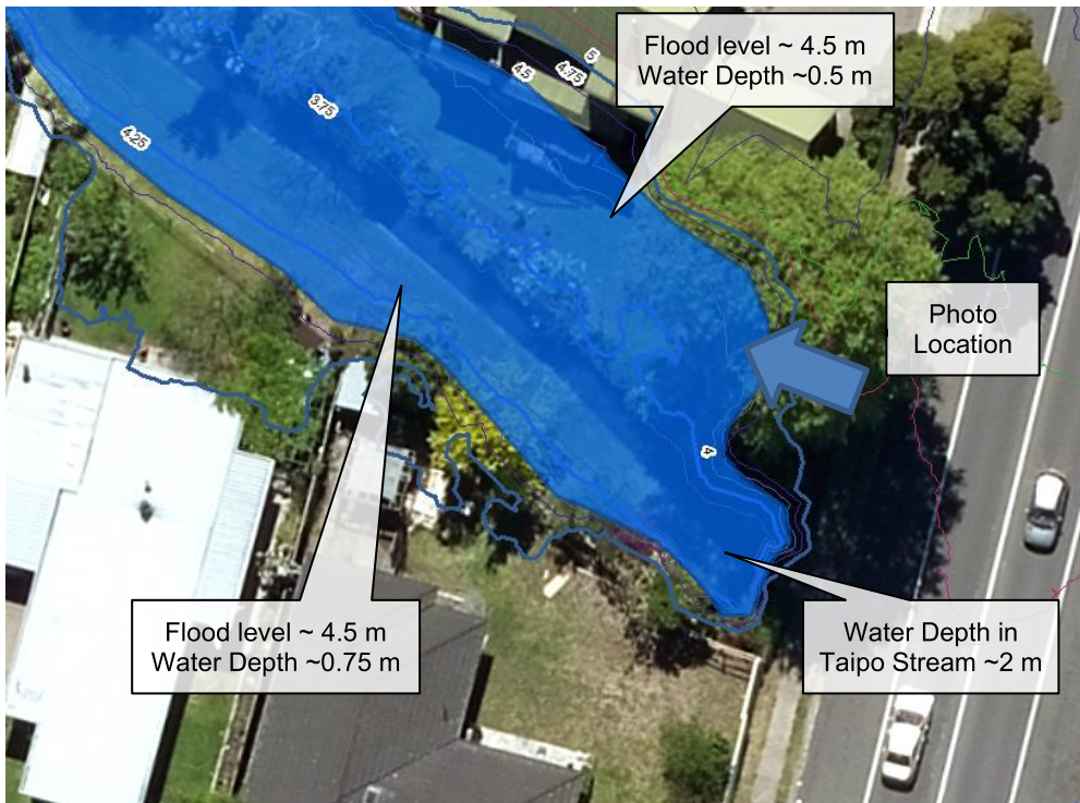
Figure 31: Taipo Stream flood extents u/s Church Road near Ngarimu Cres.
