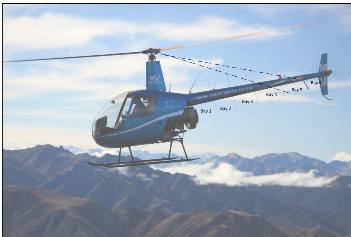
Figure 8 The tail boom impact lines
