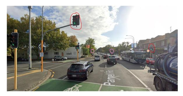
The two sets of right turn arrows (circled in red above) are green during B phase, and red in all other phases. On the phasing diagram, this is represented as the number 3 arrow.
