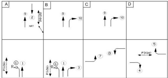
The intersection operates using 4 phases of traffic signals, labelled A to D. The phases are shown above and explained:
