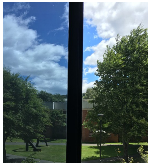
Figure 24, This shows window 1 with the low-e film on the left and the control window on the right
