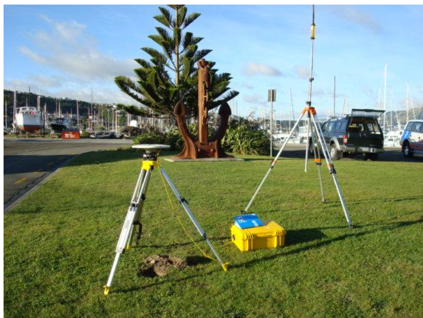
RTK Base Station at BM DML1- Entrance to Mana Marina
