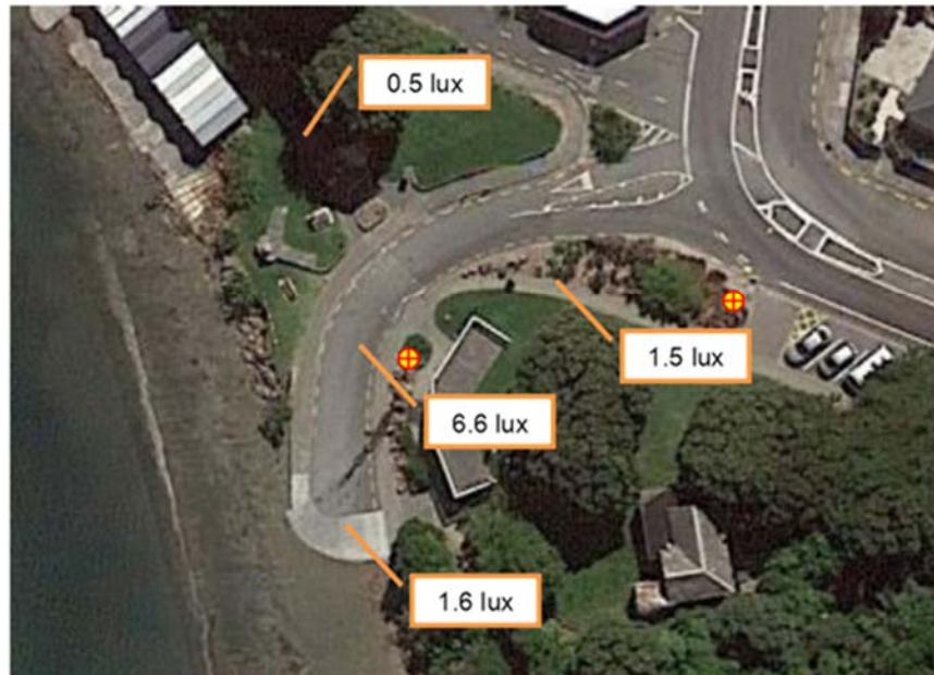
Measured Illuminance Levels
