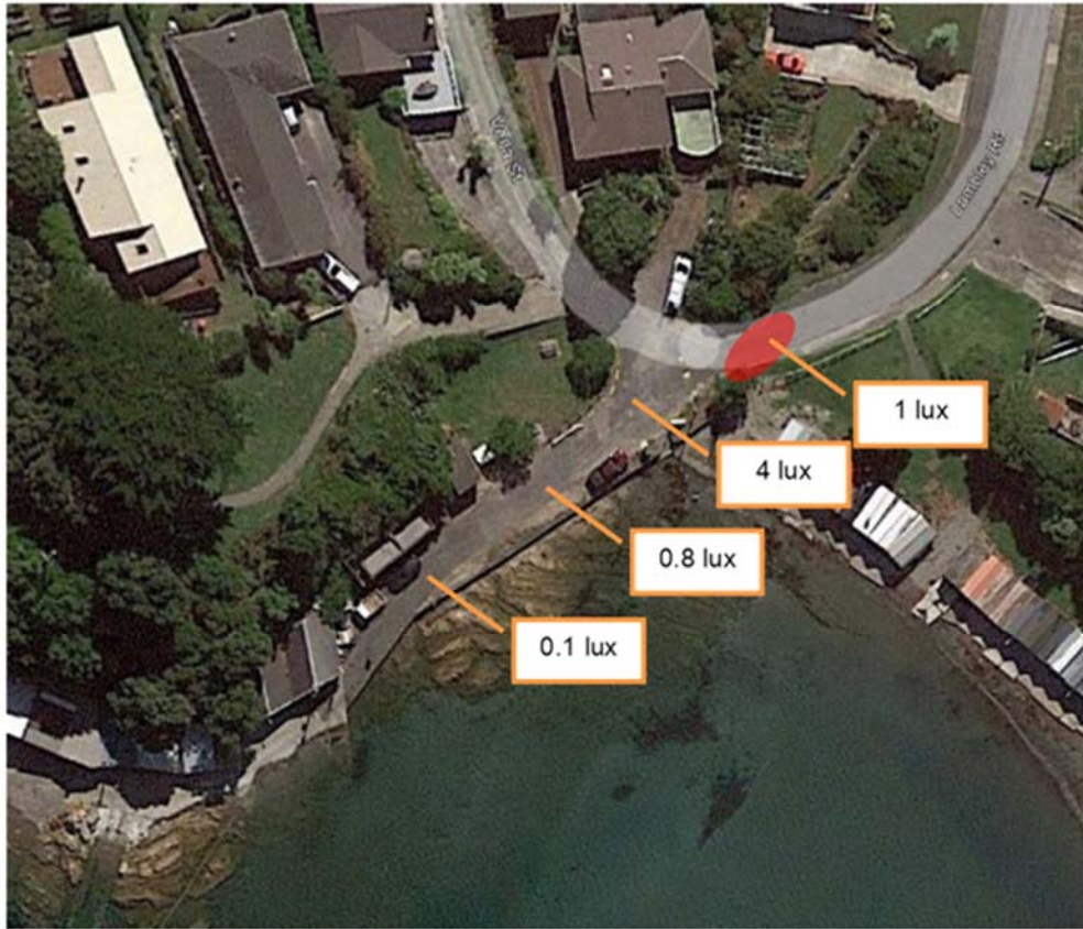
Measured Illuminance Levels
