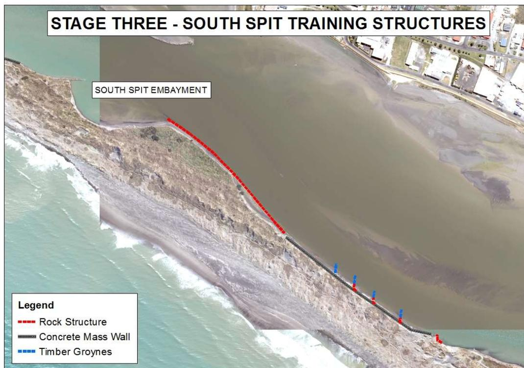
**Figure 5:** Map of the South Spit erosion protection/alignment control works.
