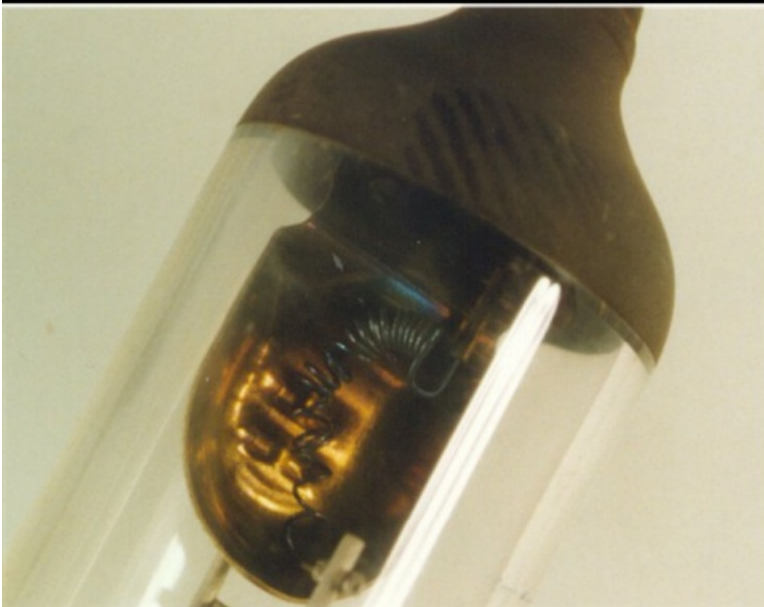
(Headlamp filament damage)
