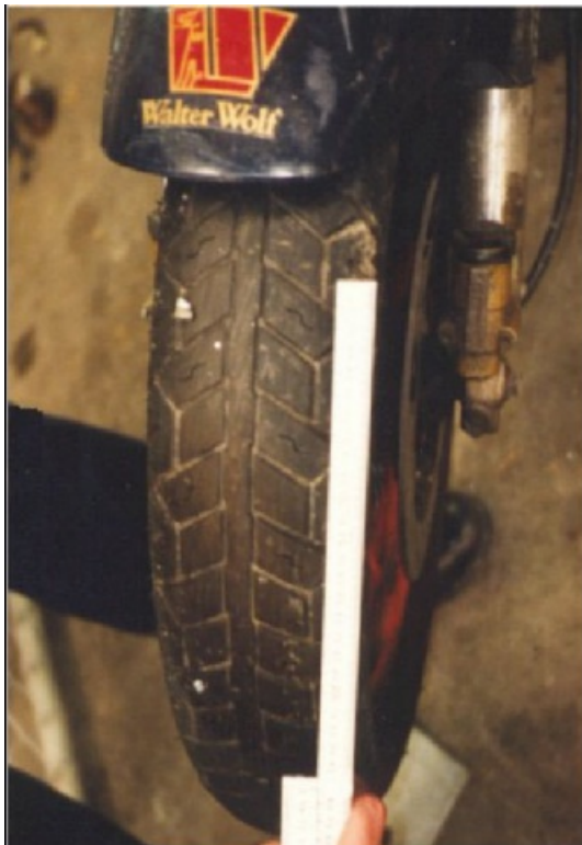
(Motorcycle front tyre shows locked wheel scuff and incipient lock up speckling)
