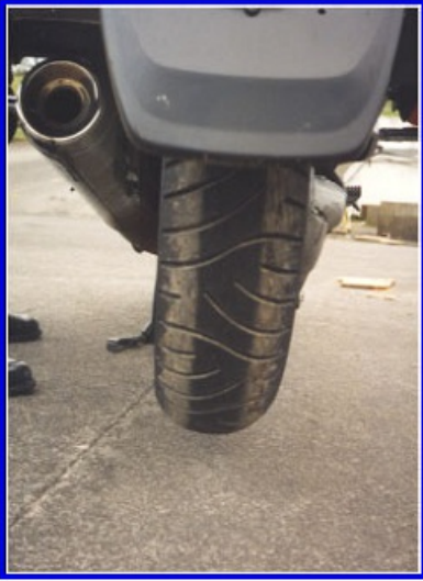
(Brake mark - rear motorcycle tyre)
