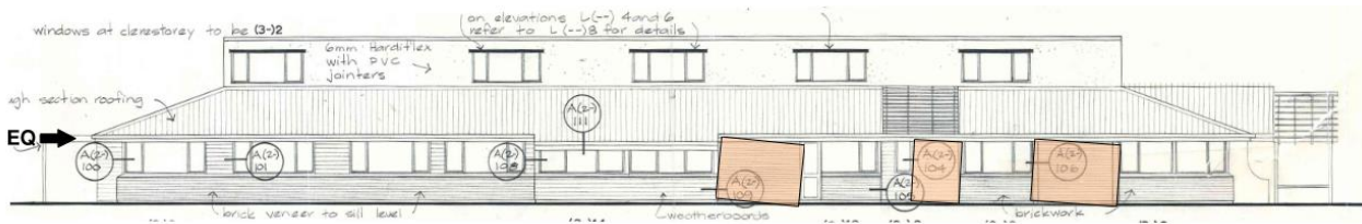
Figure 7: Typical Lateral Load Path Diagram in the NW-SE Direction (William Fraser Block SW elevation)
