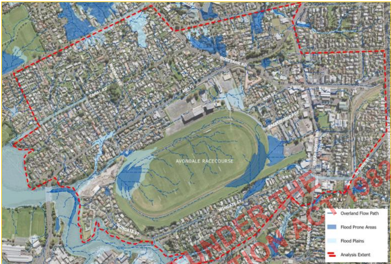
Figure 15: Flood Risks (Source: Auckland Council, November 2020)
