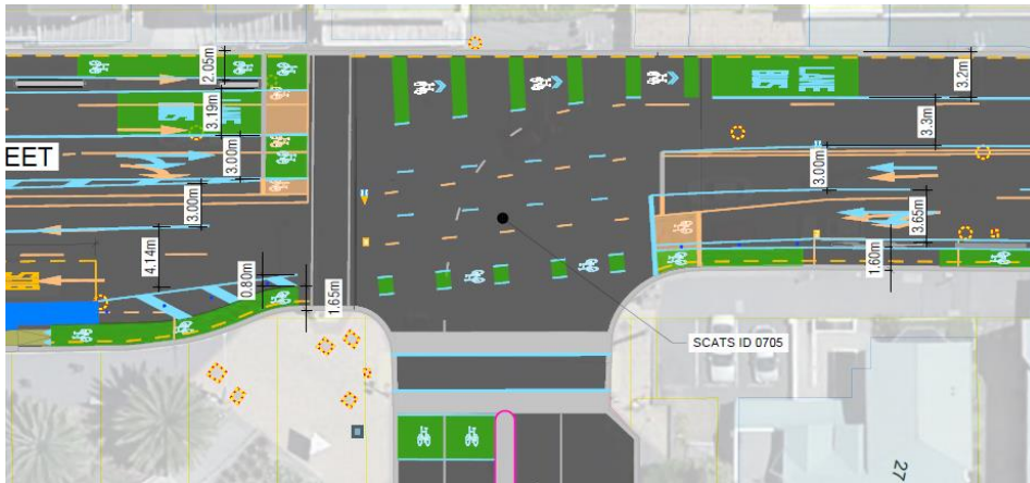
Figure 2-4: Proposed Riddiford Street / Hospital Road intersection design
