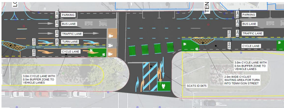
Figure 2-18: Cambridge Tce ASB at Elizabeth St intersection
