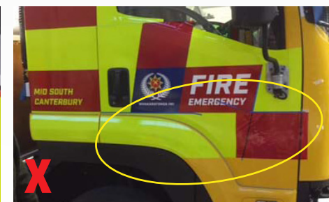
Please ensure that the Battenberg checked pattern is consistent.
