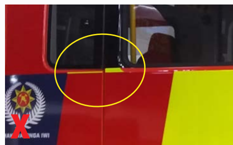
Do not apply small pieces of vinyl into areas that break the battenberg pattern.
