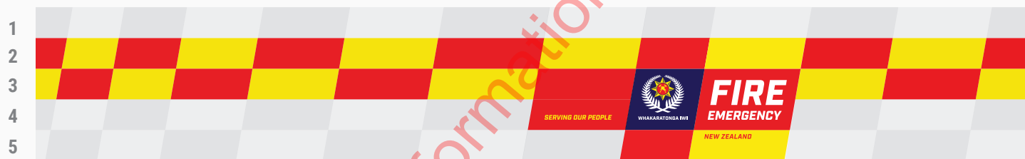
RIGHT SIDE - 'FIRE EMERGENCY' should always point to the front of the vehicle
