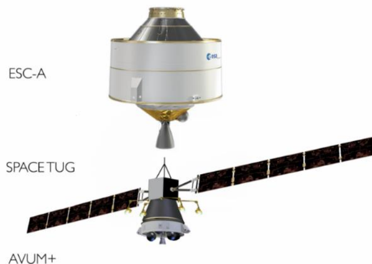
Figure 32: Vega-C based space tug design (Kochler, IRS)
