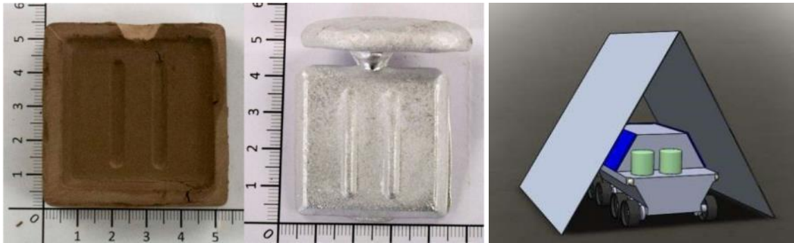
Figure 11 Regolith mould and resulting aluminium cast (“rover shelter”, Baasch, Smith, Orbit Recycling)
