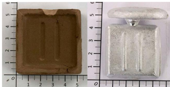
Figure 53: (Left) Sintered regolith simulant mould and (Right) resulting aluminium casting (Baasch)
