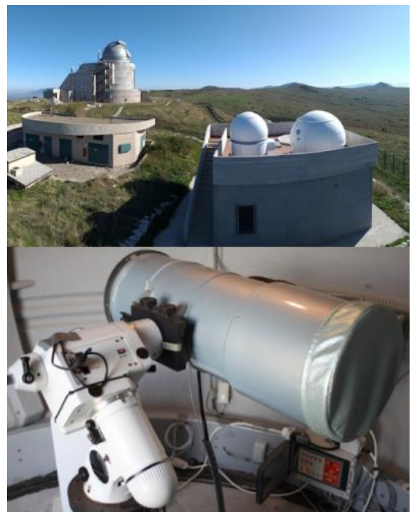
Figure 69: View of the ISON-Castelgrande Observatory (top, front) with its 2-m and 3-m domes together, and of the 22-cm telescope (bottom) of the observatory.
