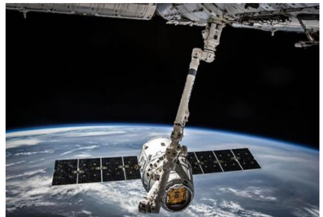
Figure 25: ISS with its CANADARM capturing a supply vessel (NASA)
