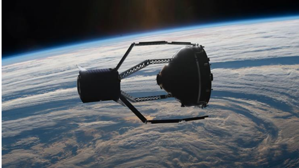
Figure 30 ClearSpace' four-arms removal concept (ClearSpace, (9))
