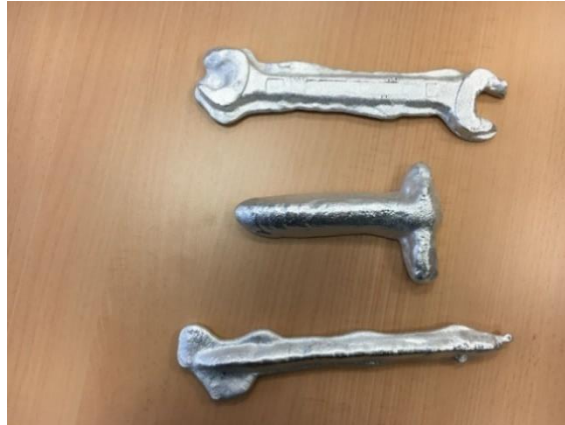
Figure 56 Tools cast out of aluminium by Lukas Schlüter (image: Orbit Recycling)
