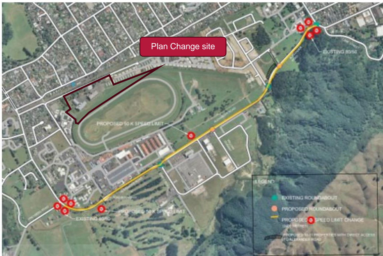
Figure 4.1 – Proposed speed limit on Alexander Road and Messines Avenue, Council’s Interim Speed Management Plan
