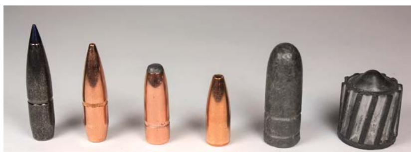
Figure 4.7. Commonly available projectile types. L-R PT, FMJ, SP, HP, Lead, 12 ga slug.
