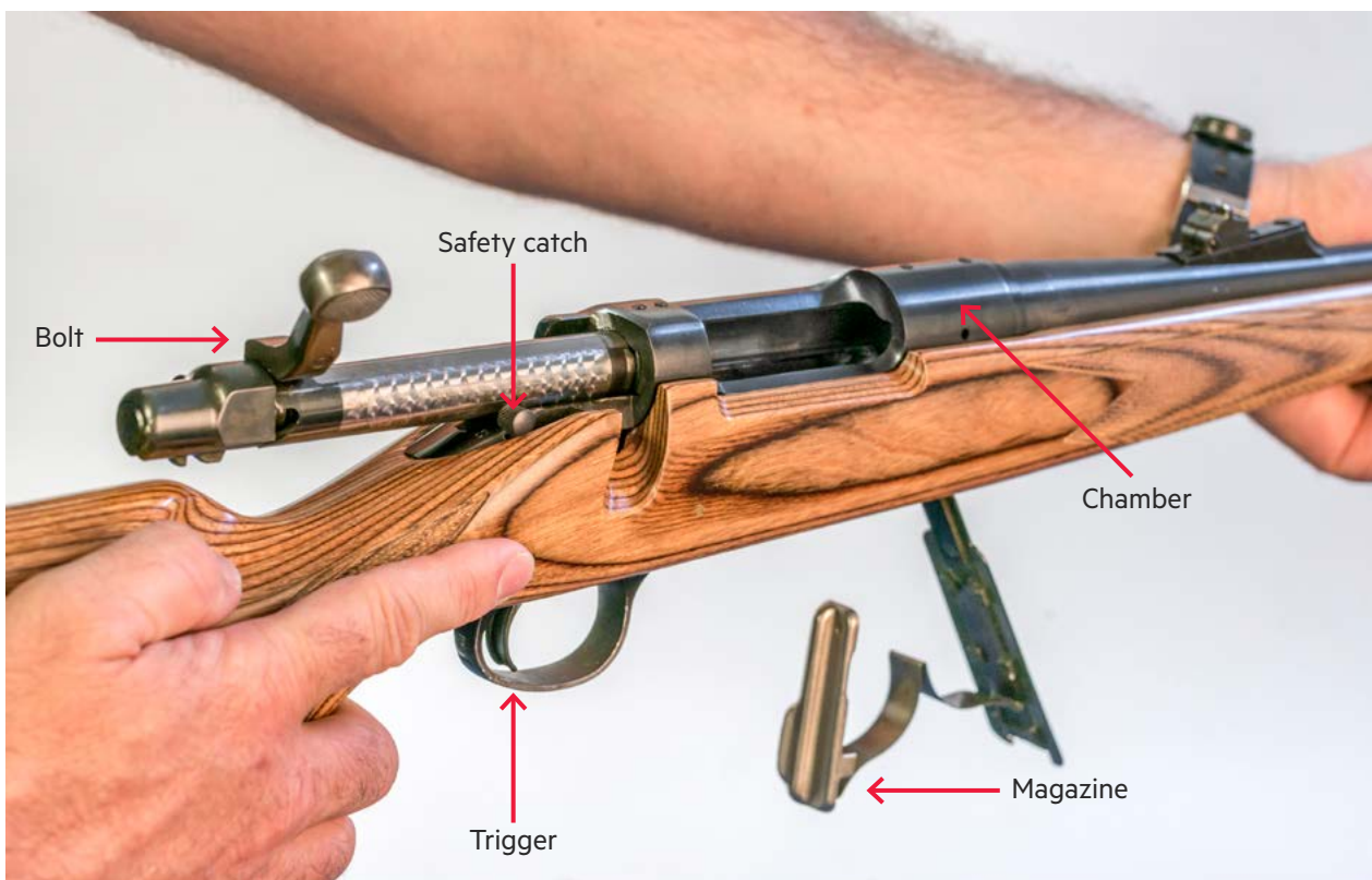
Figure 3.1. Close up of rifle action area showing common parts.
