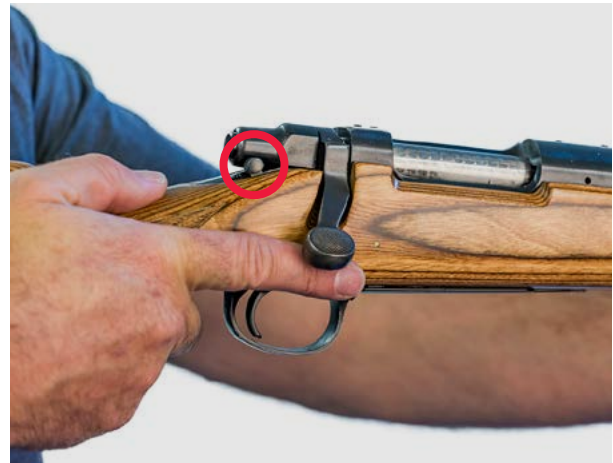
Figure 5.3. Bolt is closed on a chambered cartridge, safety catch is 'off' ('fire'), causing the firearm to be in the INSTANT state.
