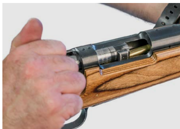
Figure 5.2. Cartridge is being inserted into the chamber, causing the firearm to be in the ACTION state.
