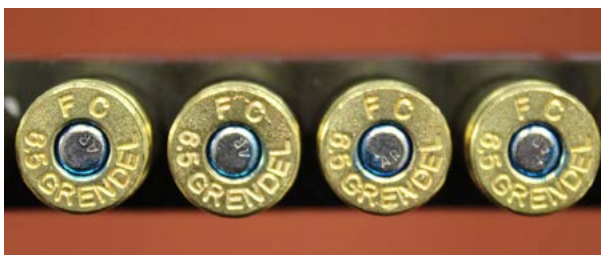
Figure 4.3. Headstamp showing calibre (6.5 Grendel) and manufacturer (FC Federal Cartridge).
