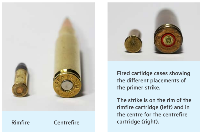
Figure 4.6. Rimfire and centrefire cartridges showing the different primer locations.
