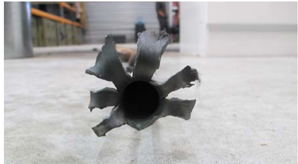
Figure 7.4. Images of a barrel damaged due to obstruction at the muzzle.
