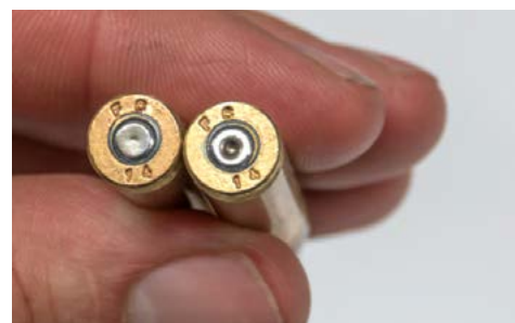
Figure 4.18. A centrefire cartridge showing: light primer strike on left, normal strike on right.
