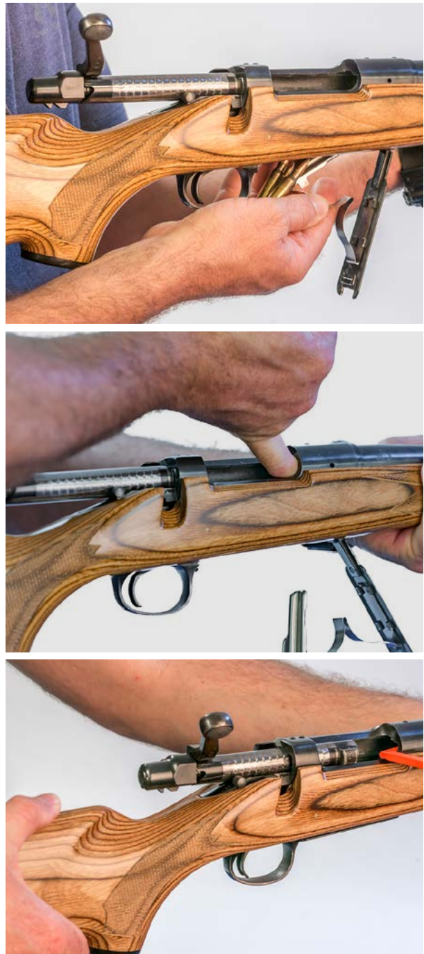
Figure 5.4. Top: cartridges removed from the magazine; Middle: physical check of the chamber; Bottom: chamber flag inserted.
