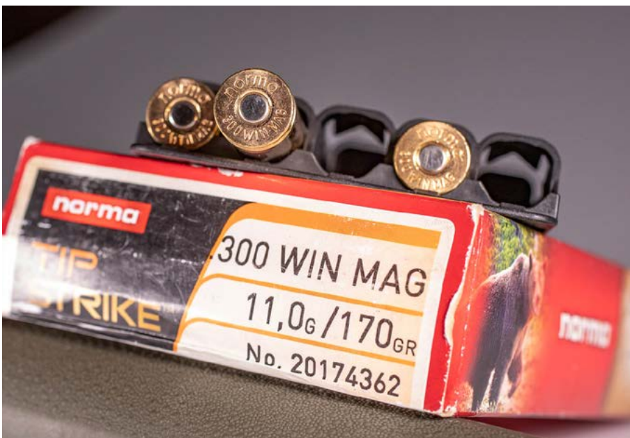
Figure 4.5. Cartridge identification information (on the box) and cartridge headstamp match.
