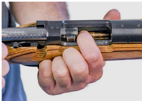
Figure 5.1. Firearm in the load state. Note cartridges are in the magazine, but the chamber is empty.
