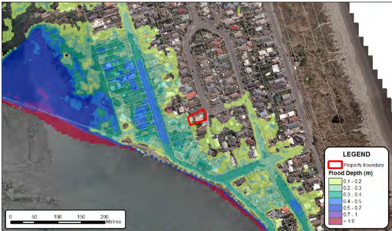
Map 3: Modelled flood depths for a 1 in 100 year flood event after the Canterbury earthquake sequence
