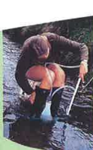
Pump sampling: Jane Halliday drives a pipe into the streambed to pump out a known volume of interstitial water along with the associated invertebrates.
