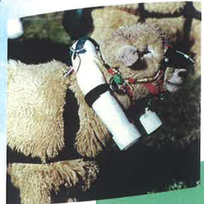
Measuring methane emitted (belched) from livestock to estimate the national annual emissions and help develop strategies to reduce them.
