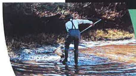
NIWA Australia staff examined the effects of road runoff on aquatic ecosystems in South East Queensland. Here, Ngaire Phillips samples macroinvertebrates in Logan River, and snail cages are set out to assess heavy metal bioaccumulation.
