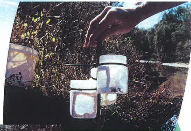
NIWA Australia staff examined the effects of road runoff on aquatic ecosystems in South East Queensland. Here, Ngaire Phillips samples macroinvertebrates in Logan River, and snail cages are set out to assess heavy metal bioaccumulation.
