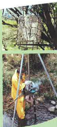
Pump sampling: Jane Halliday drives a pipe into the streambed to pump out a known volume of interstitial water along with the associated invertebrates.
