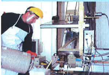
Mike Kotcamp calibrating the ozone microwave radiometer at Lauder.
