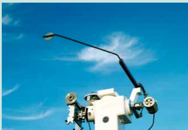
The solar tracker and instrument array measures direct and diffuse solar radiation at Lauder, Central Otago.
