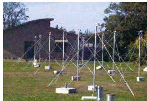
Testing the portable met stations before they were installed along the transmission line.
