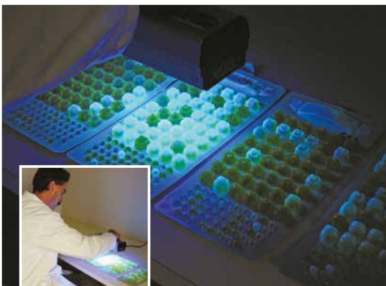
Mike Crump reading Colilert plates for E. coli.
