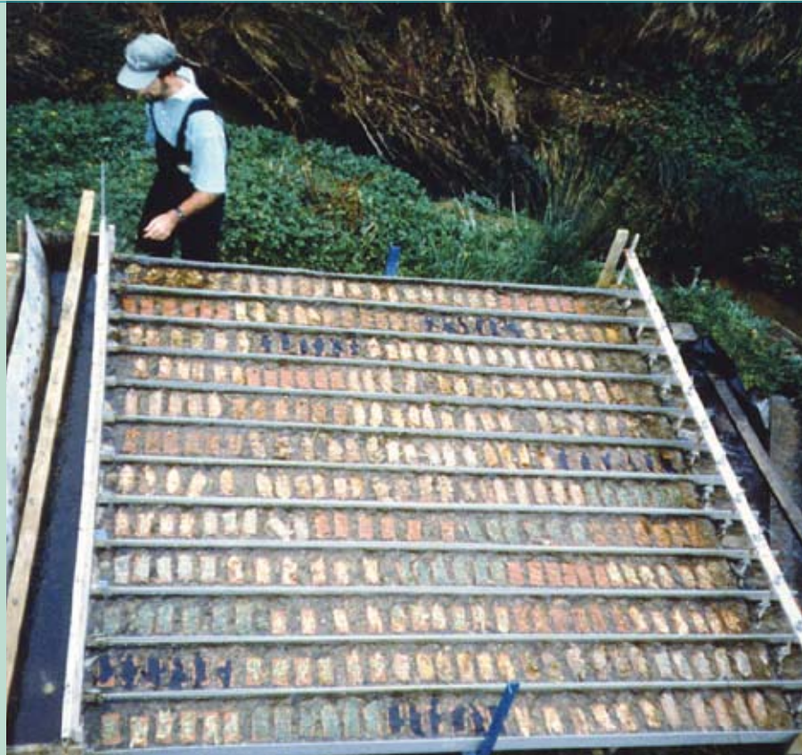
Experimental flow channels used to test the effects of various land uses on streams.
