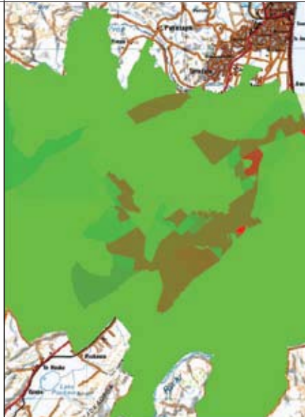
A screenshot from RiskScape showing estimated cost of damage to cars if the stopbank along the Ngaruroro River were to breach during a 1-in-50 year flood. The simulation was supplied by Hawkes Bay Regional Council. The lime green colour shows the extent of the area modelled; cars in these areas would not be damaged. The heaviest damage to cars would be in the red areas. In reality, for this scenario, there would be at least 12 hours' warning, allowing time to shift vehicles.
