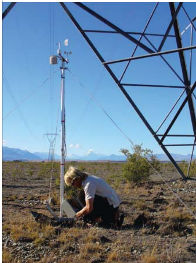
NIWA's Shane Rodwell downloads data from a portable meteorological monitoring station near Twizel during the power transmission line survey. Aoraki Mt Cook is in the distance.
