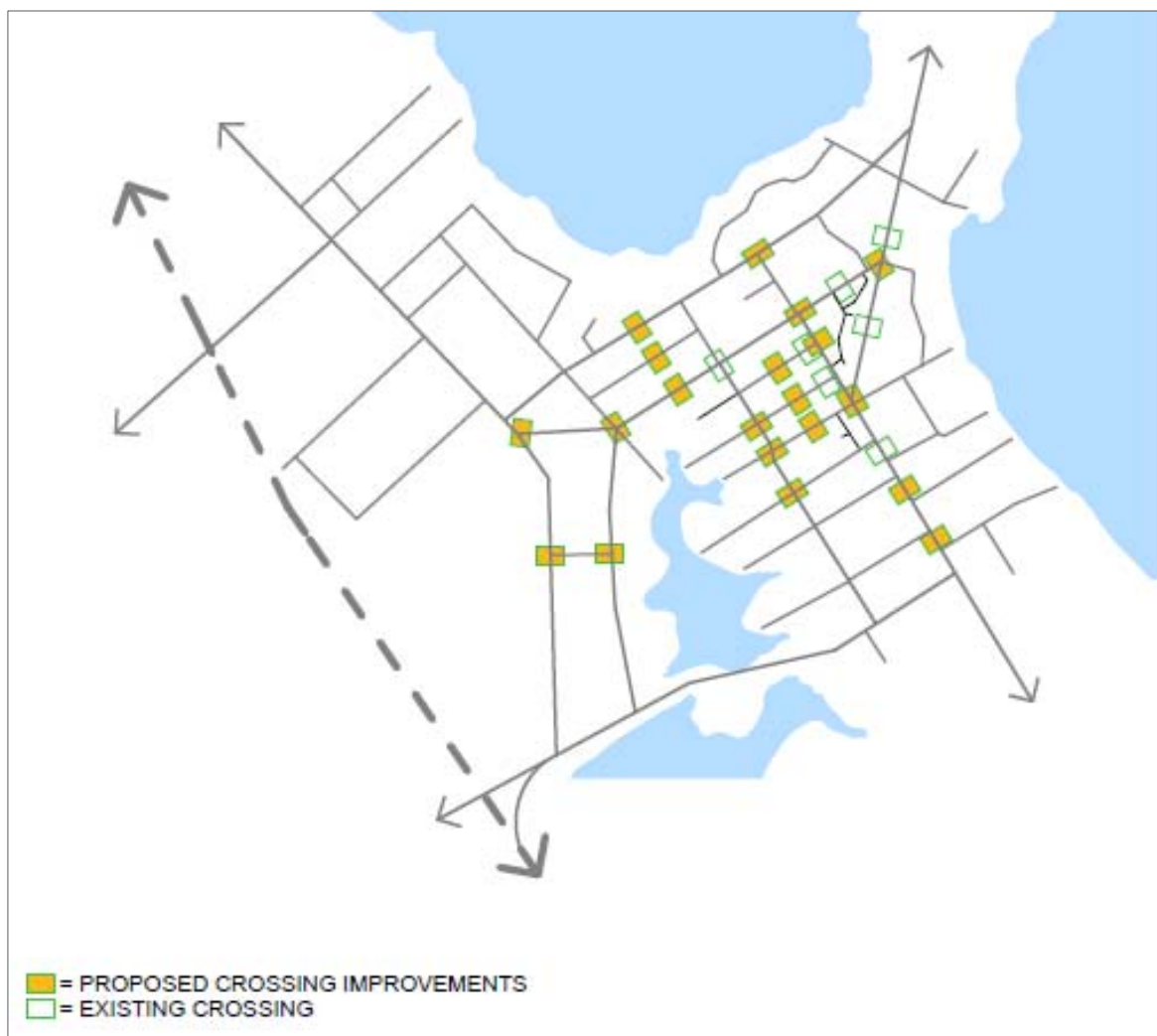
Figure 45: Existing Pedestrian Crossings and Proposed Crossing Improvements
