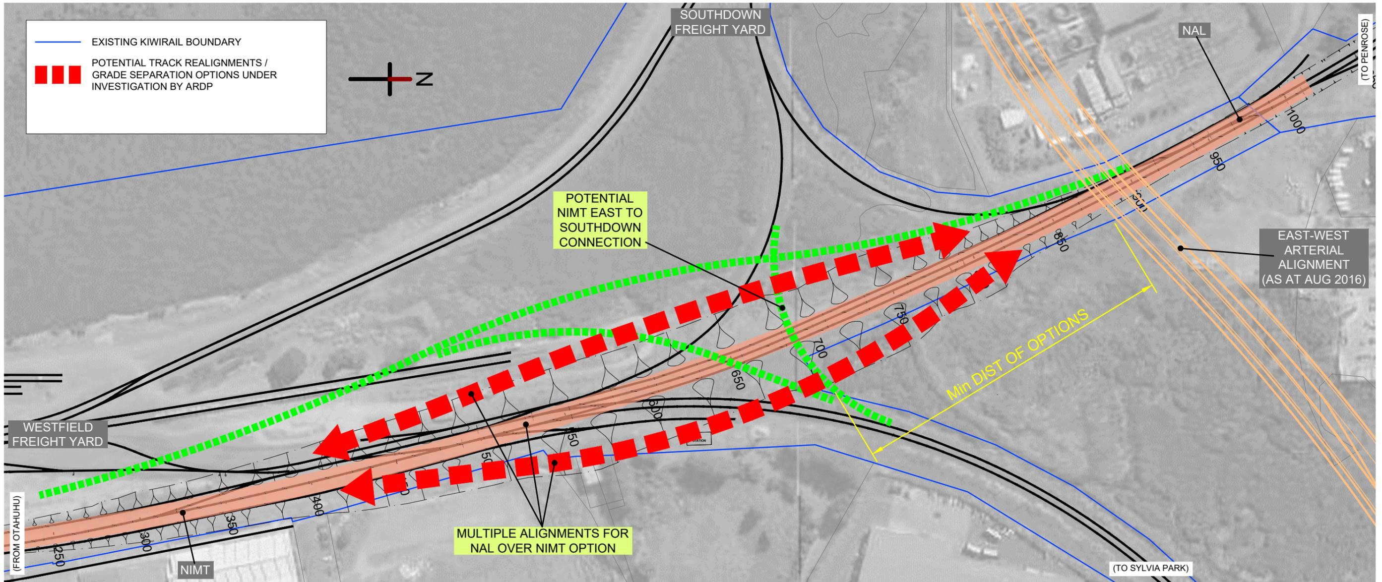
RAIL GEOMETRY IS AT MAX GRADIENT AND MIN VERTICAL CURVATURE FOR 80kph. RESULTANT CLEARANCE TOP OF RAIL TO TOP OF CURRENT ROAD DESIGN IS ~6.5m. IT IS RECOMMENDED THAT THE ROAD IS LIFTED 0.5m TO ACHIEVE ~7.0m AS FUTUREPROOFING.
