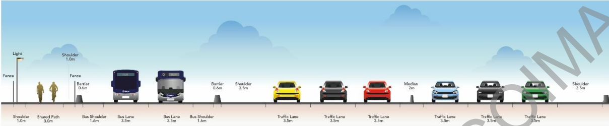
Figure 6.3 - Separated busway cross section
