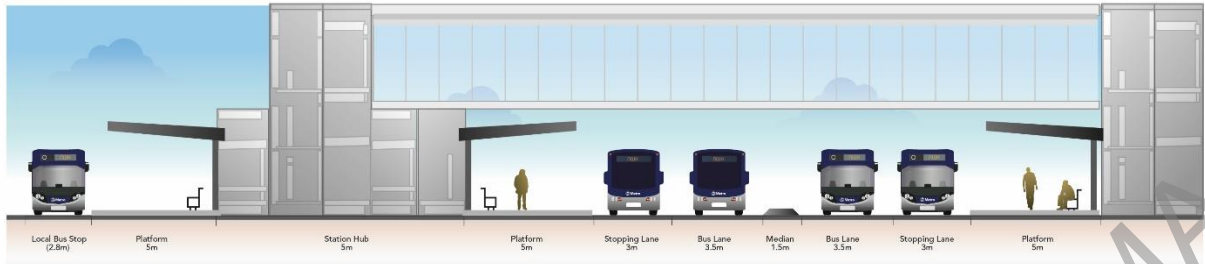
Figure 6.5 - Bus station cross section (Major)
