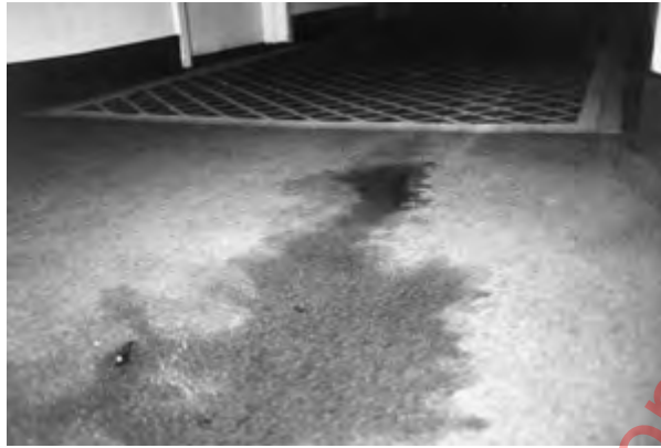
FIGURE 6.3.7.8.3(b) Irregularly Shaped Pattern on Carpet Resulting from Poured Ignitable Liquid; Burned Match can be Seen at Lower Left.
