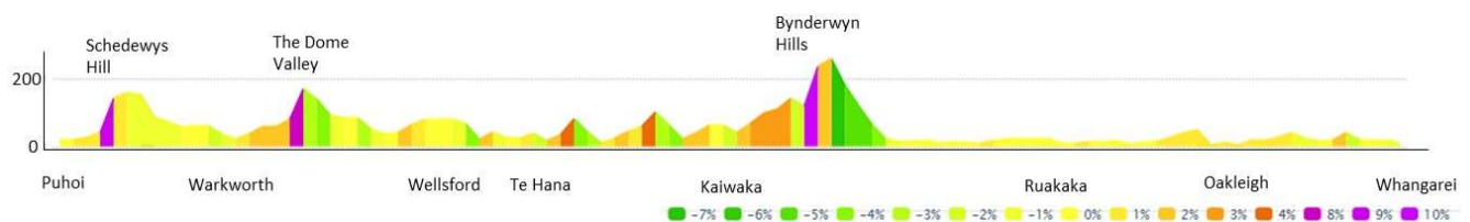
Figure 14: Vertical profile of the Auckland to Whangarei corridor
