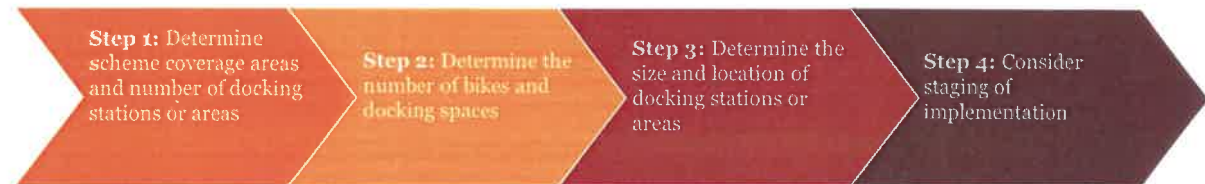
Figure 33: Method for designing the size and layout of a cycle share scheme 70
