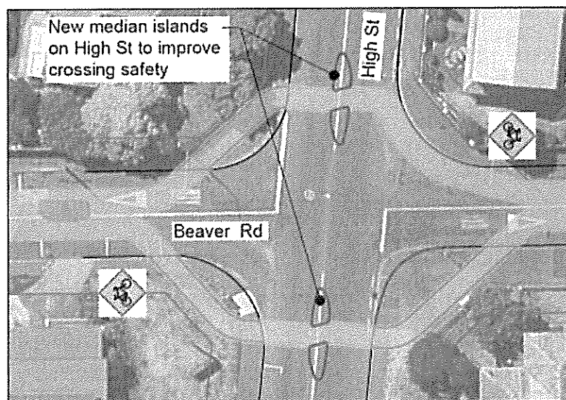
Figure 4-3: median refuges to aid crossing at High Street; please refer to full plans in Appendix B for balance of proposals along Beaver Road
