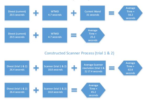
When the process steps are clumped together in the above manner, the constructed scanner process is, on average, 6.4 seconds (11%) slower than the baseline for those passengers that alarm the WTMD/Scanner. For those passengers that do not alarm the WTMD/Scanner, this constructed scanner process is, on average, 20 seconds (79%) slower than the baseline.
