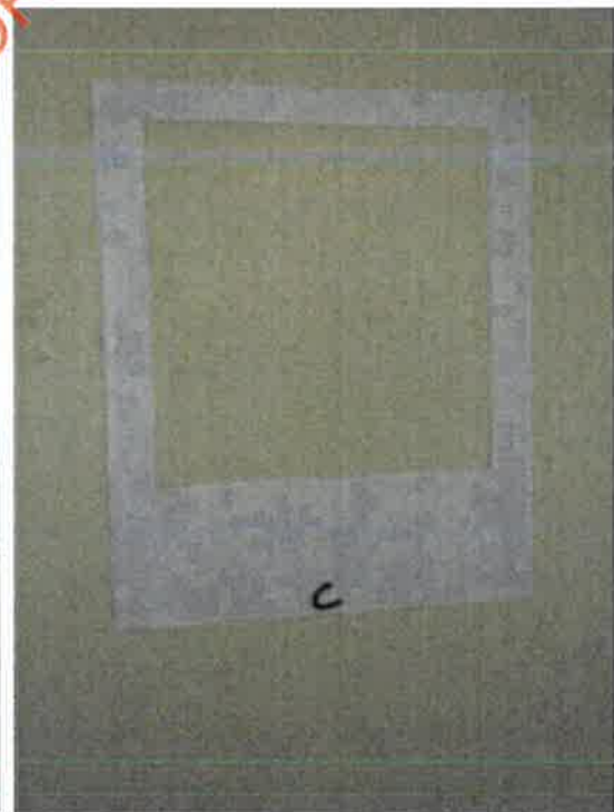
Toilet wall: methamphetamine was detected on this surface at 3.19 \mu\text{g}/100\text{cm}^2 .
