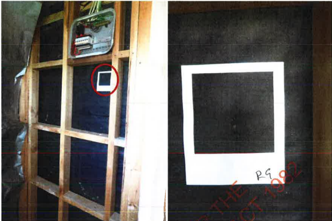
Laundry building paper: methamphetamine was detected on this surface at 0.26 \mu\text{g}/100\text{cm}^2 .
